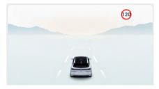
For speed limit signs categorized by vehicle type, the Intelligent Speed Assist System displays the speed limit value for small vehicles.
