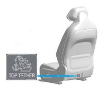
The rear passenger outboard seat position ISOFIX / i-Size lower anchors are located between the seat cushion and the seat backrest. The i-Size labels are located on the base of the seat backrest.
