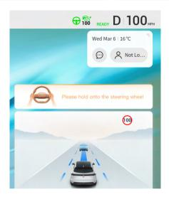
In some cases, IACC cannot be activated, such as the wiper is in high-speed gear, the lane lines are not clear, etc. Please follow the prompts on the central control display.
