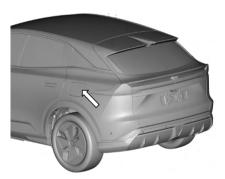
Unlock the vehicle, press the charging port cover to make it pop open, and pull out the dust cover of the slow charging socket.
