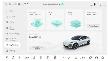
The vehicle supports two methods for detecting the overall software version: automatic and manual. When a new version is detected, the system will automatically initiate the download process.
