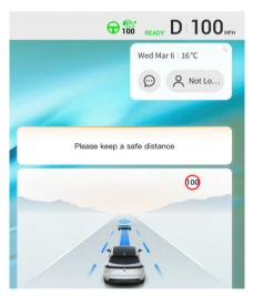
When the vehicle is driving at a medium or high speed, if there is a risk of collision with the target in front, the center control display will prompt "Risk of collision" and give a continuous sound alarm.
