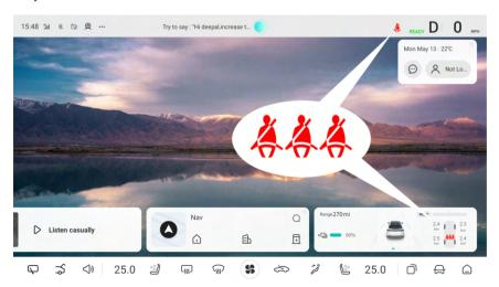
When the rear seat safety belt is not fastened while the vehicle is running, the corresponding indicator will also illuminate and a warning tone will sound at the same time. After the occupants in the rear seats have fastened their seat belts, the indicator light goes out and the warning tone disappears. While the vehicle is driving, if a seat belt becomes unfastened, the corresponding seat belt indicator light will illuminate and a warning tone will sound.
