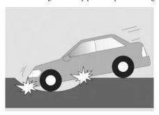
In the following conditions, even if the impact velocity of the vehicle is high, the front airbags will not be deployed. But whether they will be deployed in an actual collision must be determined based on whether the deceleration generated by the vehicle as a whole when the actual collision occurs meets the deployment conditions.
