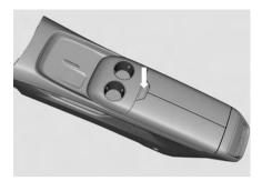
Press the button on the front of the armrest console to open the armrest console.
