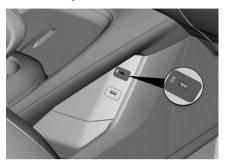
Located below the armrest box, front row users can use devices with Type-C interfaces for charging.
