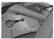
The power socket of the armrest console provides 12V DC power, suitable for appliances with power  $\leq$ 120W.
