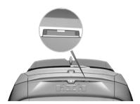
On the Bluetooth key operation page within the mobile app, tap the [Trunk] option. Lift the back door to the equilibrium position, at which point the back door will automatically open.
