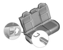
The rear ISOFIX / i-Size top tether anchor points equipped with ISOFIX / i-Size top tether anchors behind the seat backrest, with the top tether anchor identification on the seat back.
