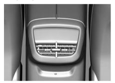
Adjust air vent: Use the up, down, left and right adjustment buttons to control the wind direction, opening and closing of the rear air vent.
