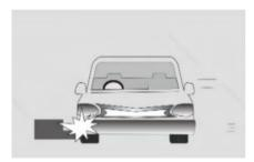
In the following conditions, even if the impact velocity of the vehicle is high, the side airbags will not be deployed. But whether they will be deployed in an actual collision must be determined based on whether the deceleration generated by the vehicle as a whole when the actual collision occurs meets the deployment conditions.
