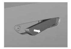
The electric retractable door handle automatically extends when the vehicle is unlocked. Pulling the handle will open the door.
