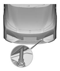
The front towing point is located below the right side of the front bumper. Open the tow hook cover and screw in the tow hook to use it.
