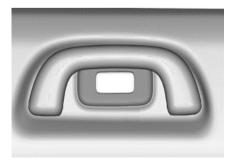
The rear reading light can be turned on and off by pressing the lens.
