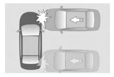
When a vehicle sustains an angled impact from the side, the intrusion speed into the vehicle's side is relatively slow.
