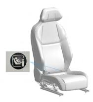
The front passenger seat is equipped with ISOFIX / i-Size top tether anchors behind the seat backrest, and at the base, with the top tether anchor identification at the base. It is necessary to lift up the seat cover when using it ×.
